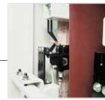
Belt oscillation controlled by an electronic photocell for longer lifespan of the belt.
