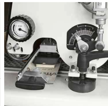
ON/OFF PNEUMATIC SELECTOR FOR COMBINED UNIT It allows the roller exclusion, or the sanding pad exclusion or both of them, from the sanding process while maintaining the working table position unchanged.
