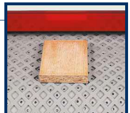
Natural rubber vacuum table with diamond-shaped belt: the best piece traction and the maximum stability.
