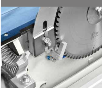
Device for the blade micro-lubrication Compulsory for the machining of light alloys, extremely useful with particular plastic materials.
