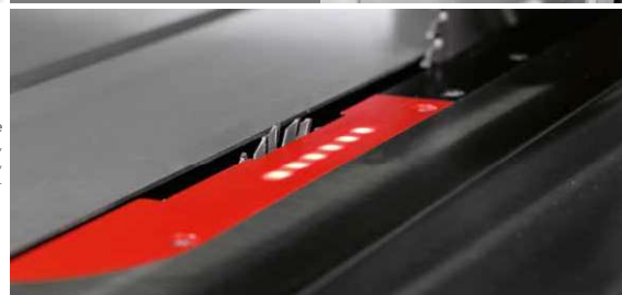
"LED indicating scoring unit in operation" device When the scoring blade is working, the high efficiency LEDs clearly indicate the danger area, making the machine safer than ever.
