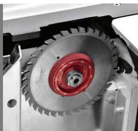
Expandable scoring blade Manually expandable with variable thickness from 2,8 to 3,6 mm. Blade diameter: 120 mm (160 mm for class si x)
