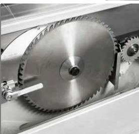
"Pro-Lock" System for the main blade rapid locking with fast and tool-less riving knife adjustment.
